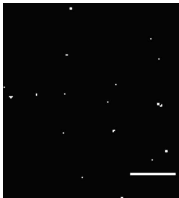
Fig. 3. EFM fluorescence image of DNA tetrahedron nanolabels on the substrate. Scale bar 10 \mu\text{m} .
